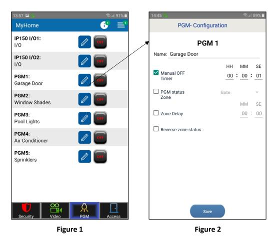
Note: The IP150 PGMs are shown only if configured as outputs (inputs not supported)
