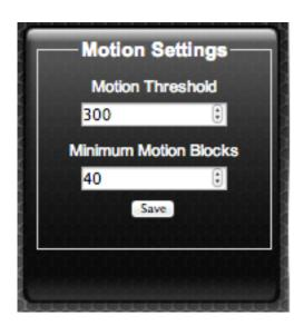
Motion Threshold - changes the sensitivity of the alarm system. 100 high sensitivity. 900 very low sensitivity. We generally start with a setting of 200.
